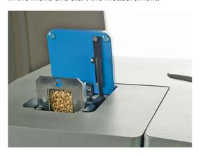
Fill the grain into the shaft, choose the analyzed product in the menu and start the measurement.
